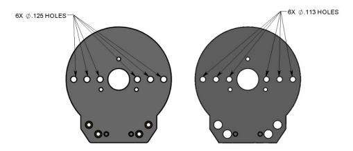
Figure 1, Small-bore bases side by side showing new hole sizes (left) and current design (right)
