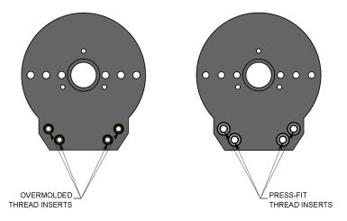
Figure 2, New (left) and current (right) threaded inserts
