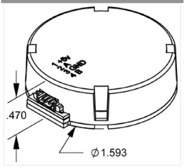
Cover Extension (E-option) provides space in the cover for longer shafts up to 0.836":
