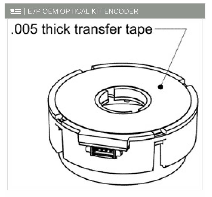
The **T**-option base provides a transfer adhesive (with peel-off backing) that may be used when mounting holes are not available. A centering tool is required when using this option.
