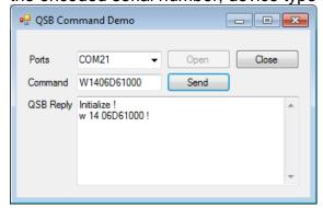
Step 13. To verify the firmware version, click the Close button then click the Open button. When a new connection is opened with a QSB device, it responds with QSB-[device type] [version]! as shown below.
