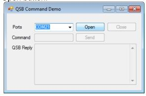
Step 9. If the device has not been initialized, then a dialog will prompt for the device serial number. Enter the serial number which can be found lasered on the top of the QSB device.
