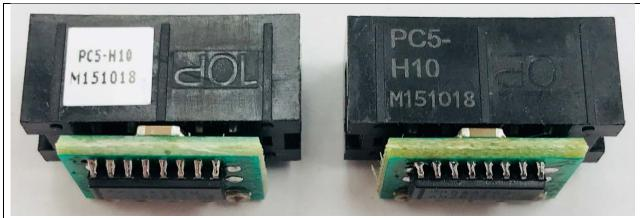
Side-by-side comparison of the current PC5-H10 labeling (left) and the new PC5-H10 laser marking (right).
